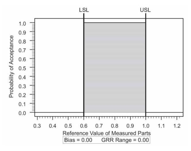
Figure IV-F 1: Gage Performance Curve Without Error
