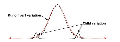
When this process is studied in production with the production gage, more variation (i.e., a smaller Cp) will be observed. For example, if the *GRR* of the production gage is 30% and the actual process Cp is still 2.0 then the observed process Cp will be 1.71.
