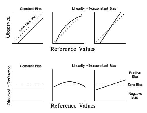
Possible causes for linearity error include:
