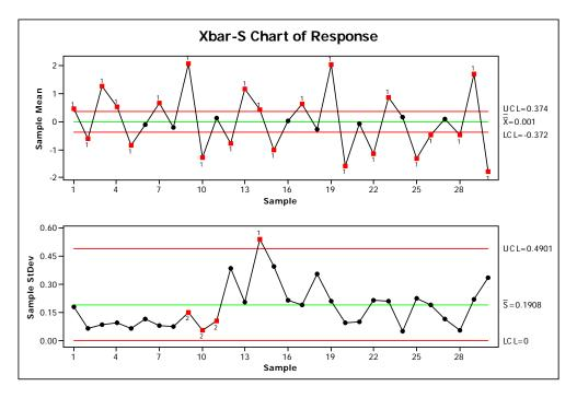
Figure IV-H 1: Pooled Standard Deviation Study Graphical Analysis<sup>80</sup>
