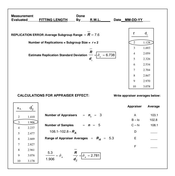
Figure IV-E 3: Alternate Computations for Evaluating a Measurement Process (Part 1 of 2).
