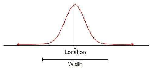
Figure I-E 5: Characteristics of the Measurement Process Variation
