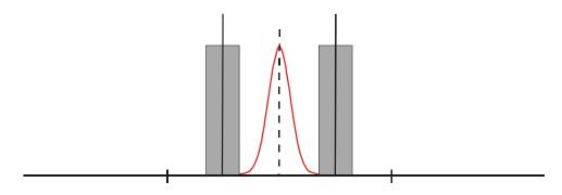
Figure III-C 3: Example Process with *Pp* = *Ppk* = 1.33
