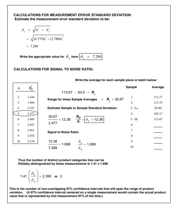
Figure IV-E 4: Alternate Computations for Evaluating a Measurement Process (Part 2 of 2).
