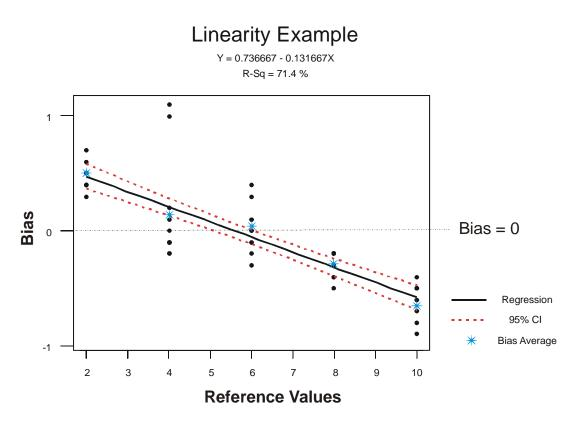
Figure III-B 3: Linearity Study – Graphical Analysis
