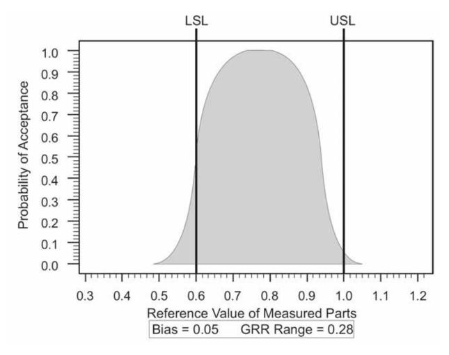
Figure IV-F 2: Gage Performance Curve – Example
