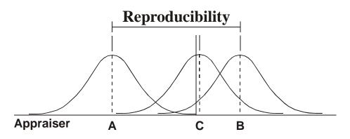
The ASTM definition goes beyond this to potentially include not only different appraisers but also different: gages, labs and environment (temperature, humidity) as well as including repeatability in the calculation of reproducibility. Potential sources of reproducibility error include:
